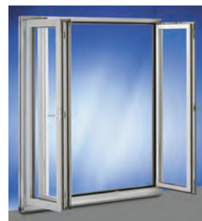
Folding sashes moved to the side to form a slim package. Fold and Slide units are equipped with an optional Tilt and Turn passage (in-swing or out-swing) door. In the secured tilt position, this sash can be used for ventilation.
