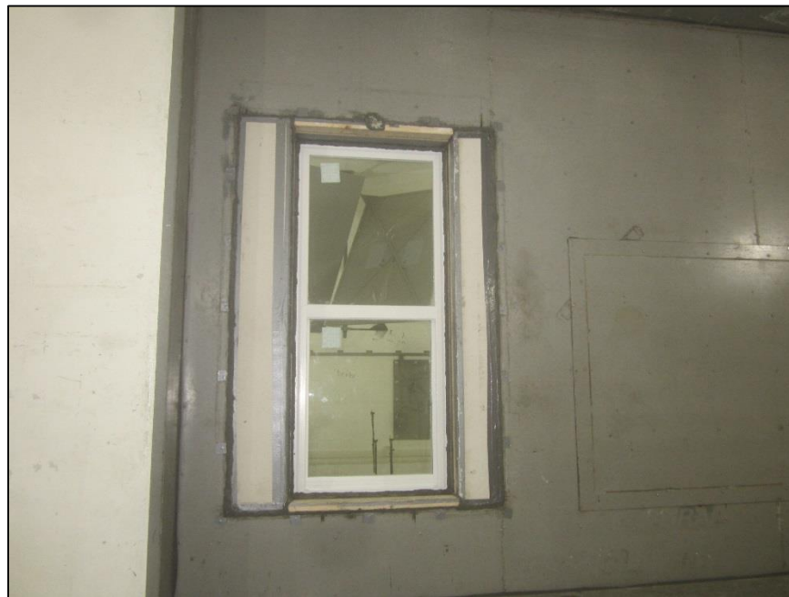
Source Room View of Installed Specimen
