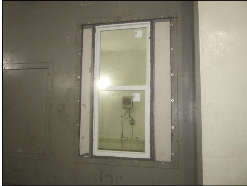
Receive Room View of Installed Specimen
