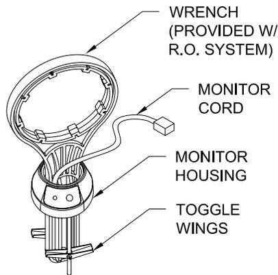
4. Place the Toggles of the Monitor Housing Assembly through the mounting hole on the sink or counter top.
