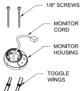
3. Feed the Monitor Cord through the 1¼" diameter Monitor Housing opening so that it is positioned above the Monitor Housing.
