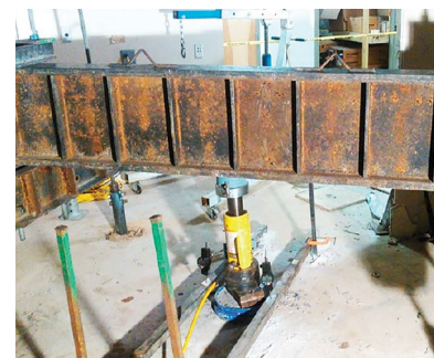
Compression load test setup
